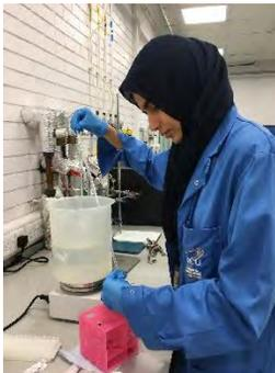
*Extracting NIPAAm hydrogel polymer solution after dialysis*
