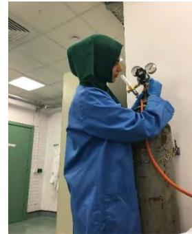
*Setting up nitrogen gas cylinder for Nitrogen Purging*
