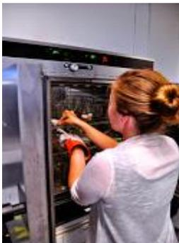
*Working with the drying oven to prepare the palm leaf sample*
