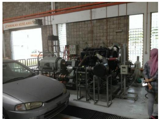
*Diesel test engine setup at the CAREM*
