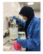
Extracting NIPAAm hydrogel polymer solution after dialysis
