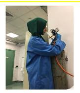
Setting up nitrogen gas cylinder for Nitrogen Purging
