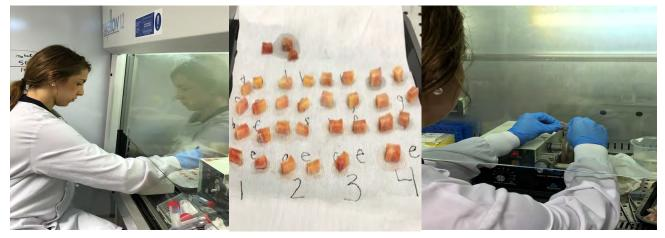
Here I am using a slow-speed diamond bladed saw to cut through a femoral bone sample into the square pieces.
