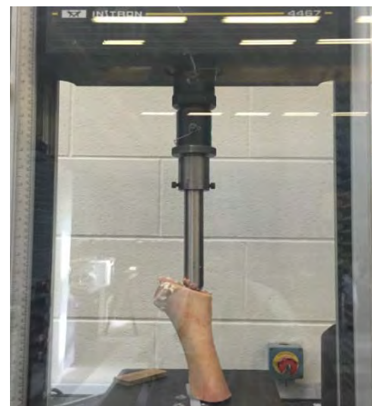
Insertion of machined hip implant into bovine femur using Instron 4467 compression testing machinery.
