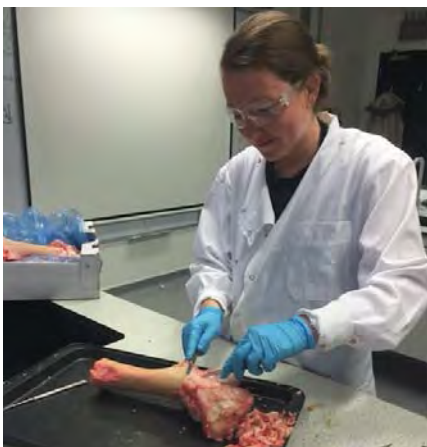
Preparing bovine femoral samples for mechanical testing.
