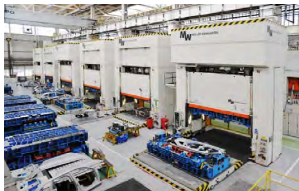
Some of the presses used to test the stamping dies
