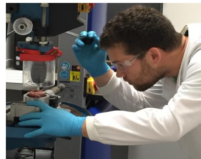
Isolating Trabecular Bone Cores from Ovine Vertebrae. The bone cores were then implemented into a Bioreactor.
