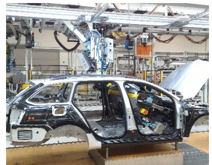
One of Škoda's many moving assembly lines. This factory produces over 2,300 cars per day.
