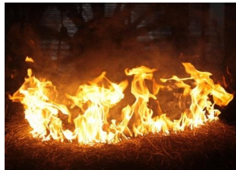
Close-up view of fire propagation. Wind speed: 1 m/s, Angle: 10°
