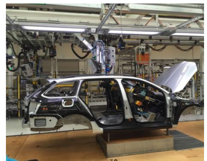
A Skoda Octavia in the process of being built in the factory
