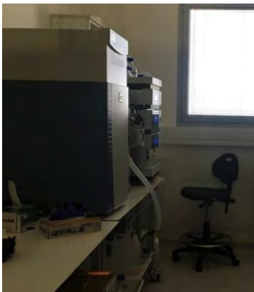
Mass Spectrometry machine used to analyze metabolites
