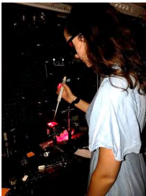
Using a pipette to place the sample solution on a glass prism for testing.
