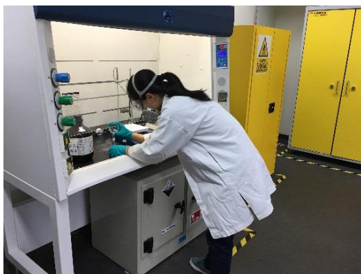
Measuring the amount of chloroform necessary to make a membrane
